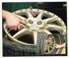
The hub is a precise fit in the rim, and so a little gentle persuasion may be required to separate the two - using only a soft-headed mallet
