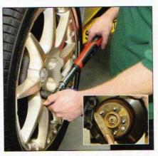
To avoid possible seizure of wheel to hub in the future, both mating faces are cleaned and coated with copper-based grease before re-fitting. Re-balancing is not usually required as the rim, wheel centre, and tyre have not altered their positioning in relation to one another
