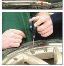
The Schrader valve itself is hidden deep within the wheel rim, and is unscrewed to deflate the tyre
