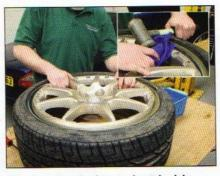
Next the wheel centre is sat back in place, aligning the inflation hole with the valve recess - it can be gently adjusted if necessary so that everything lines up exactly
