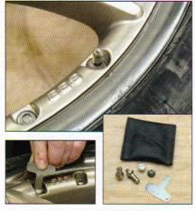
The air valve is cleverly hidden below a hollow bolt; this toolkit contains an inflator adaptor, blanking plug removal tool and spare plugs
