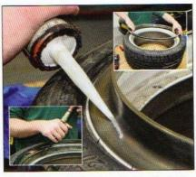
Silicone adhesive is applied to the back of the replacement trim, before fitting to the wheel rim. The bolt holes are then blown clean with compressed air, as any debris or blockage may lead the rim to split or the threads to strip when the bolts are tightened
