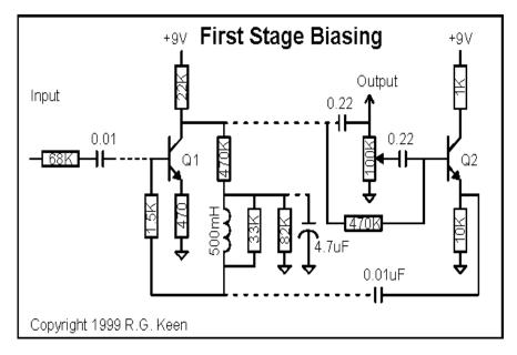
If we just guess that the collector is sitting at 4.5V, that gives a collector current of about 200uA, an emitter voltage of about 0.1V, and a voltage at the base of 0.6V roughly. The voltage across the 470K is then 4.5V - 0.6V or 3.9V, and the current through it is about 8uA. If the gain of the transistor is around 200, then Ib is 1uA, and the voltage across the 82K resistor is 0.6V for a current of about 7uA. Hah! An approximate match!
