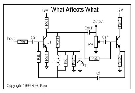
From our earlier tear-down report, we know that Q1 is a voltage gain amplifier, and that Q2 is an emitter follower that just buffers the signal voltage from the wiper of the Wah pot, Rw. We know that the inductor is fairly passive, and only participates by setting the L side of the LC filtering. Let's take a look at every part, with some comments on what the parts do and what happens when they change.
