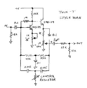
discernable. The control resistor is just a variable resistor to ground.
