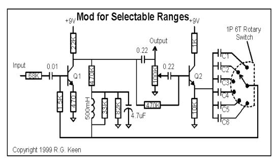
Install a switch to select between different values of Cf. Smaller values move the sweep range up, bigger values move the sweep range down. You can use any kind of switch. A SPDT will give you two choices, a 1P6T switch as shown will give you six choices.
