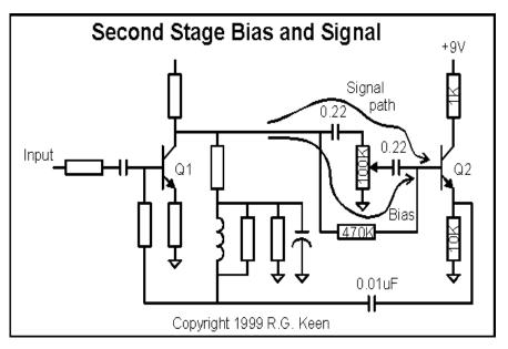
This emitter follower buffers the signal from the wiper of the wah pot, which is simply a volume-control-style voltage divider to ground. The emitter of the transistor connects through a 0.01µF capacitor to the junction of the inductor and the 1.5K resistor to the base of Q1. How the devil do you get a moveable frequency resonance out of that?
