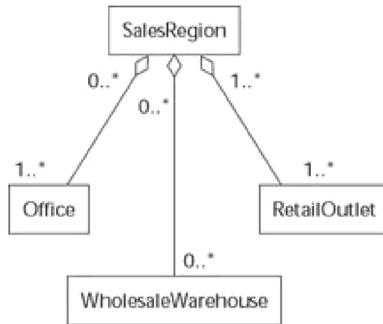
Figure 5-2: A weak form of aggregation—some parts survive if the whole goes away.
